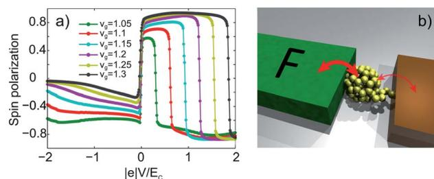
**Fig. 4** The two terminal device operation: (a) shows the spin polarization as a function of the bias voltage for different values of  $v_g$ . These are the cross-sections from Fig. 3b. The spin polarization highly exceeds the polarization of the ferromagnetic lead and it reverses sign for positive bias voltages. Panel (b) presents the proposed realization with asymmetrically coupled molecules.
